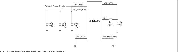
Figure 1. External parts for DC-DC converter
